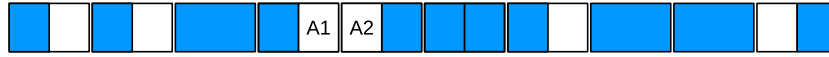
Fig. 7. Fragmentation reduces usable space. For ease of analysis, VCA has a constraint that adjacent free type A slots in neighbouring type B slots (such as A1 and A2) cannot be merged and used for allocating type B blocks.
