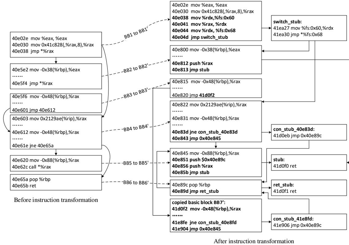
**Figure 5: An example of instruction transformation by  $C^3$ .**  $C^3$  rewrites indirect and conditional branch transfer instructions to jump to a stub (bold), and the stub will then jump to the real targets.  $C^3$  transforms basic blocks with multiple entries ( $BB4$ ) by copying each entry to a new address ( $BB4'$  and  $BB7'$ ).
