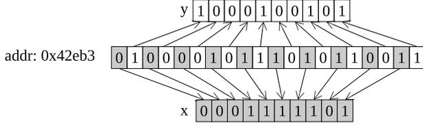
Figure 3: Extracting  $x$  and  $y$  for address  $0x42eb3$ .  $C^3$  obtains  $x$  and  $y$  from the lower-order odd- and even-index bits of an address.
